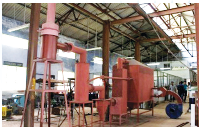
Fig. The Fabricated prototype the wax removal device
