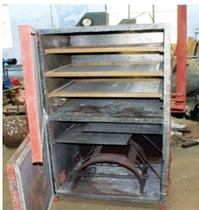
Fig. Fabricated prototype of the Biomass drier
