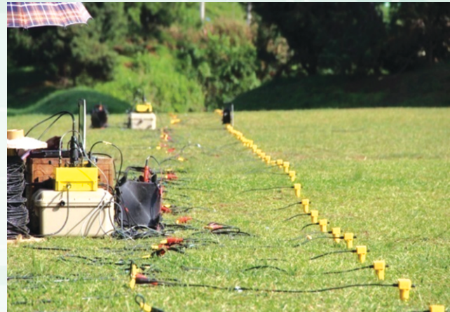
Figure : (Left) Members of field trip for MASW study along with the Professors & students of Physics Department of St. Edmunds College at the St. Edmunds College Play Ground. (Right) The layout of the instruments for multichannel seismograph system at Golf Link, Shillong.
