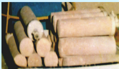
Filter- candles developed at NEIST
