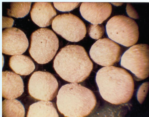
High Strength Proppants - enlarged view
