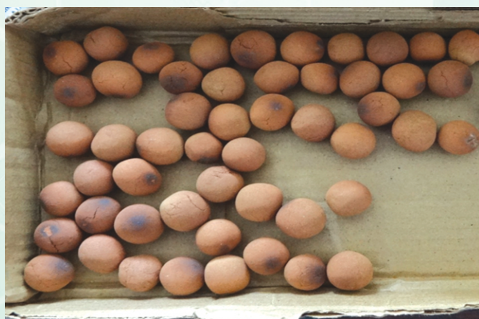
Fig Burnt Ceramic Filters Made out of Local Materials for Defluoridation of Water
