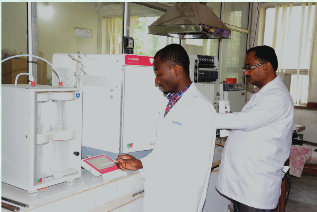
Fig: M/S Milestone Italy model flex SYNTH state of the art microwave synthesis system which consists of a single microwave platform which in combination with specific accessories, allows classic glassware and high-pressure synthesis as well as solid-phase reactions. The advanced system has been installed for the first time in the country.
