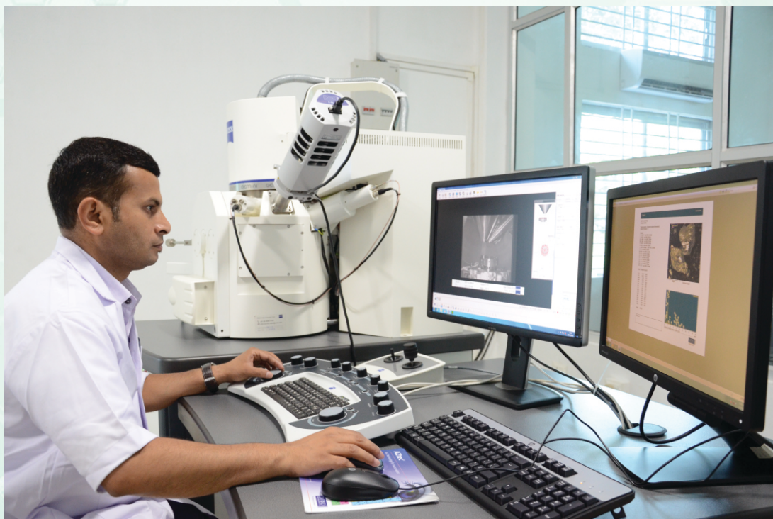
Fig: M/S Carl Zeiss make Field Emission Scanning Electron Microscope with EDS facility (FESEM with EDS)
