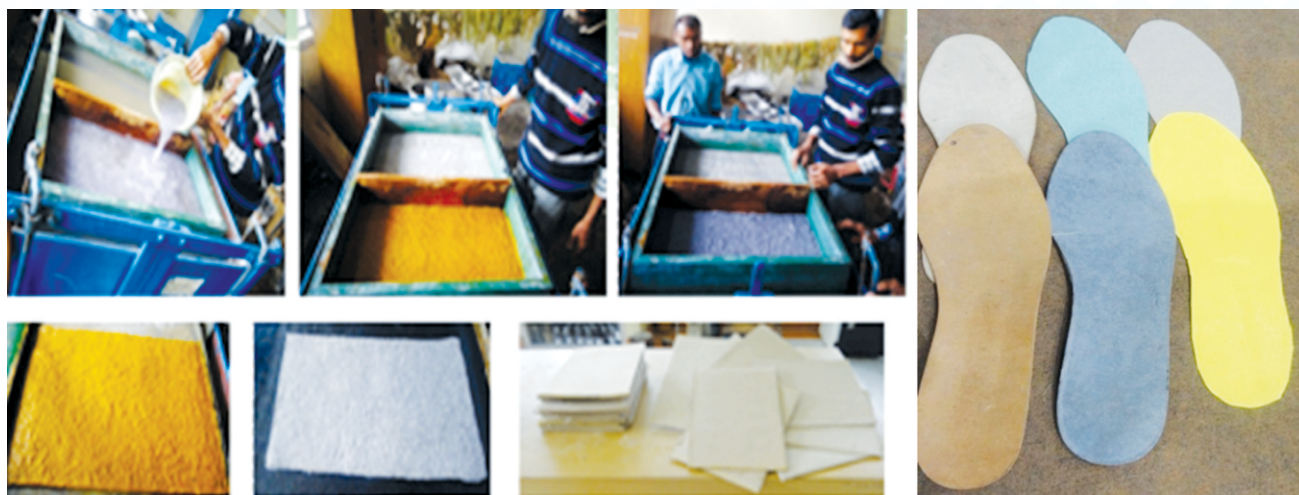
Diferent stages of board making from the mixture of El shaving and natural fibre
