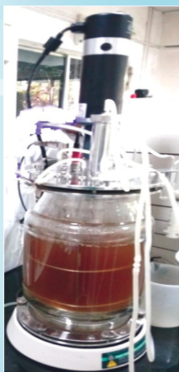
Fig : Scale-up at 10L NBS Bioreactor
