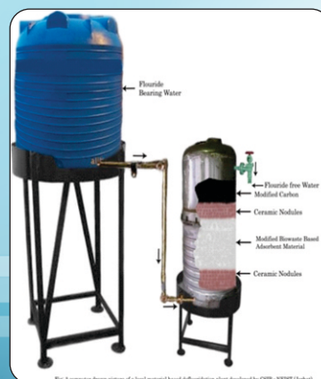
Conceptual design of the prototype to be set up in the Fluoride affected areas
