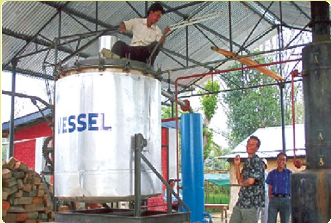
A distillation plant for citronella/lemongrass/patchouli set up by Mr Bito Luhu at Chumukedima, Dimapur
