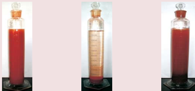
Fig. A typical snapshot showing (a) dispersed phase (b) flocculation/settling of suspended particles in 1% DP of slime slurry in the presence of natural hard water and (c) stable dispersed phase of 25% iron ore fines using water from 0 and 0.05% humate.
