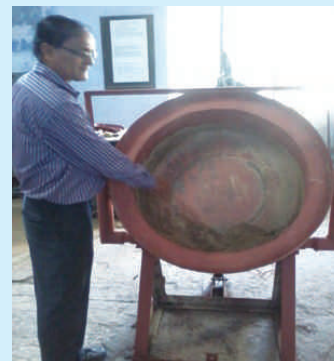
Fig.: Nodulizer Pan for Agglomeration Technology
