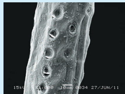
Fig.: SEM of Chemically modified Coir Fibre
